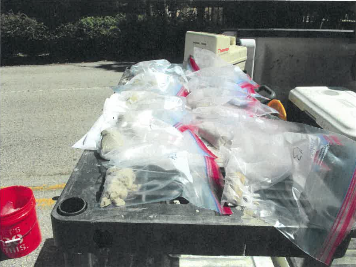
Photograph 8: View of bagged soil ready to be tested with the PID meter (instrument in the background).
