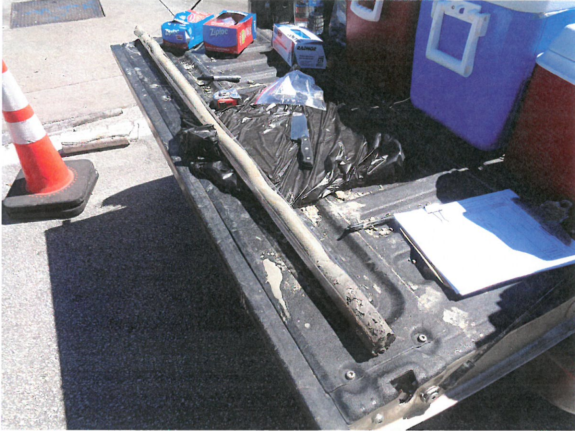
Photograph 7: Retrieved soil core in acetate sleeve ready for logging and sampling.
