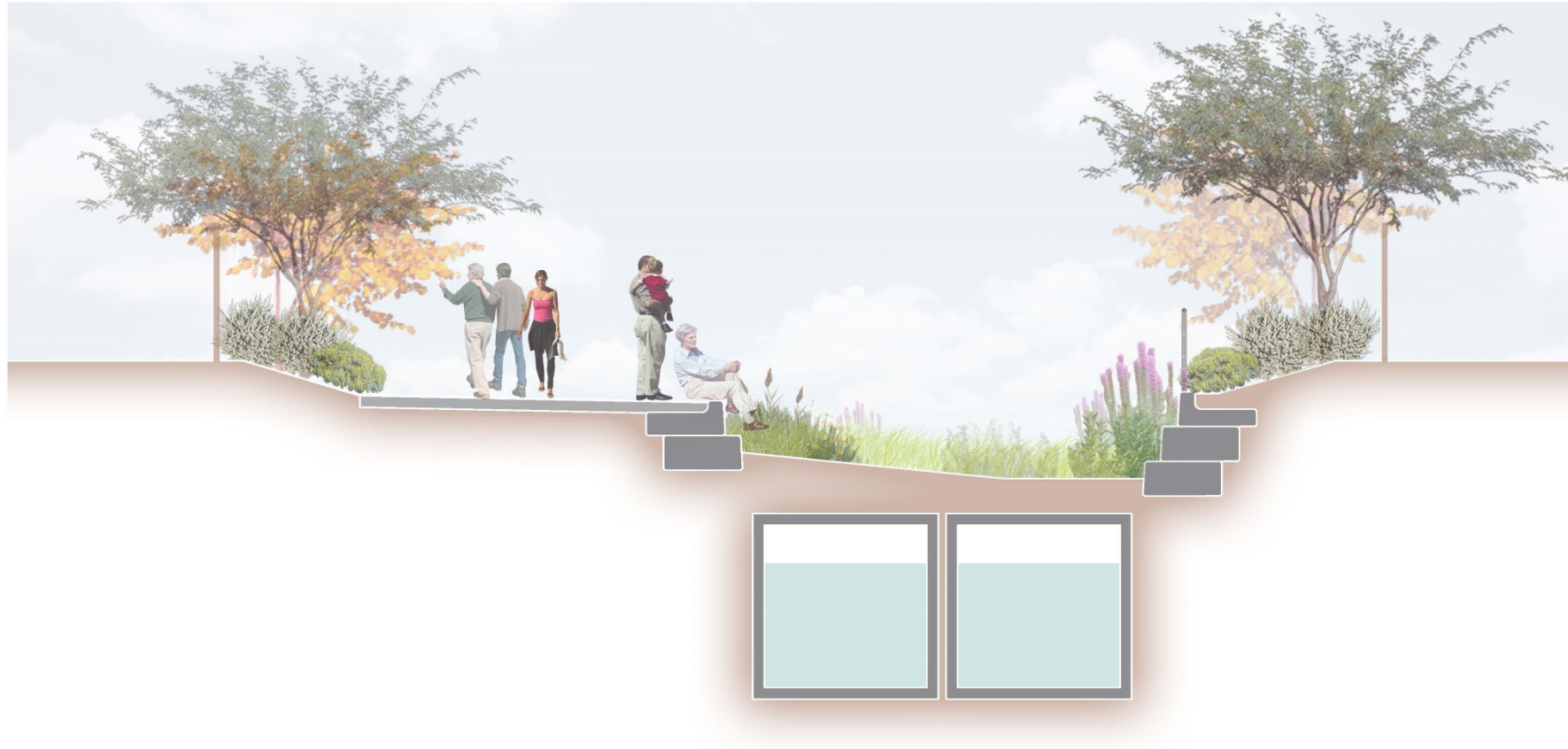
ALTERNATE E: STORM SEWER BOX ENCLOSURE
